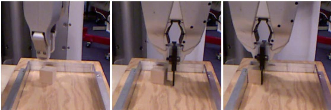
**Figure 1-1: Robot arrangement task.** *Real robot reliably assembling an arrangement. First the robot places a block, then pushes it using a paddle.*
