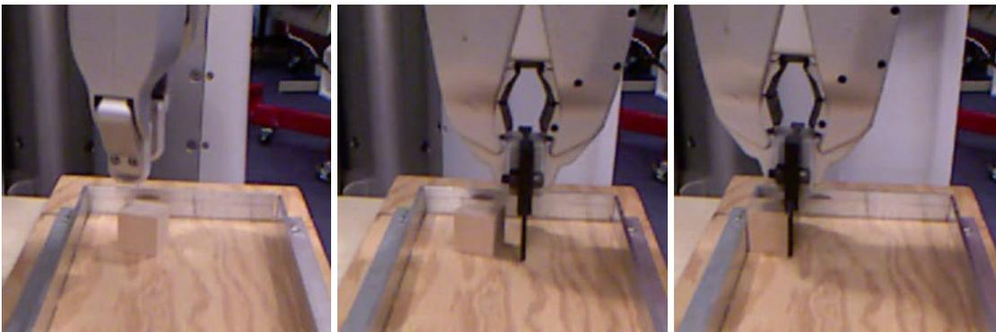
**Figure 3-10: Real robot reliably assembling an arrangement.** *These are a sequence of photographs of a robot constructing an arrangement. First the robot places a block, then pushes it using a paddle.*
